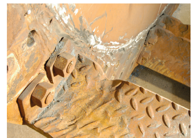
Unprotected steel fan blades showed severe erosive wear after three months of service
