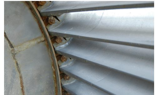
Kennametal Conforma Clad® blades on fan Unit 8B showed 0.014" after seven months run time
