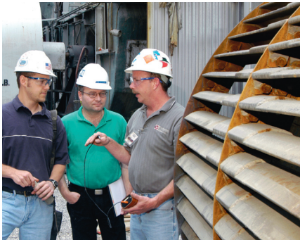
Tungsten carbide cladding measurement taken by TVA ER&TA group
